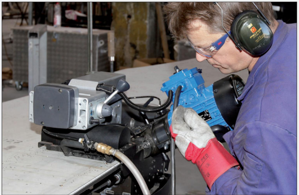
The AutoCUT 500 with automatic forward and return
