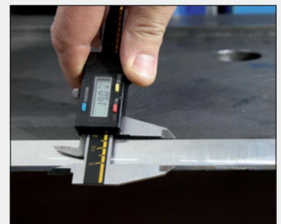
Chamfer width 30 mm max.
