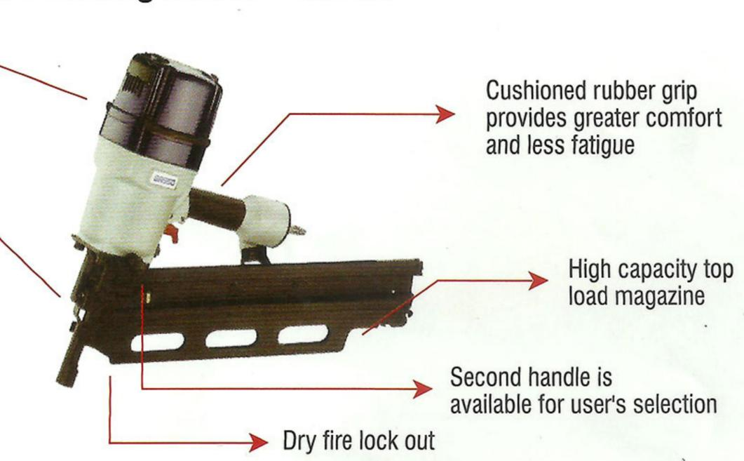
A22/160~A1 Model Fasteners 3.8 - 4.6Diameter (mm) **Fasteners** 100 - 160 Length (mm) Weight (Kg) 6.91 Operating 80 - 120 Pressure (psi) Fastener 56 Capacity  $L \times W \times H (mm)$ 568x187x538
