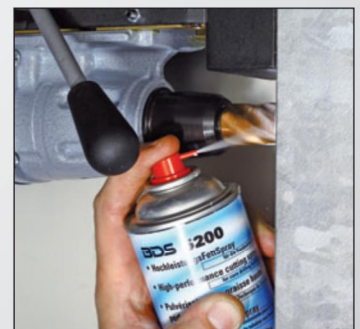
Step 2: During drilling, spray the high-performance lubrication spray onto the tip of the drill and into the borehole.
