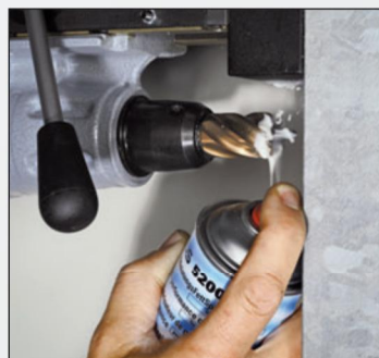
Step 1: Prior to drilling, spray the high-performance lubrication spray directly into the drill.
