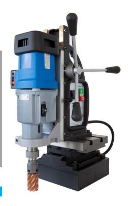
Versatile and powerful drilling machine with magnetic baseand equiped with BDS MAB 800 machine. This model is an "essential machines for general use" in engineering workshops. The machine is equipped with a powerful 4- speed drive with adjustable spindle speed, adjust the electronic control unit of the magnetic field, the cross-table, reverse, motor soft start, overload protection, automatic coolant.
