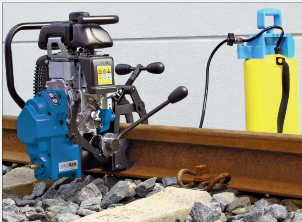
Rail MAB 600 with petrol engine. Performance 1.5 kW, torque 3.04 Nm.
